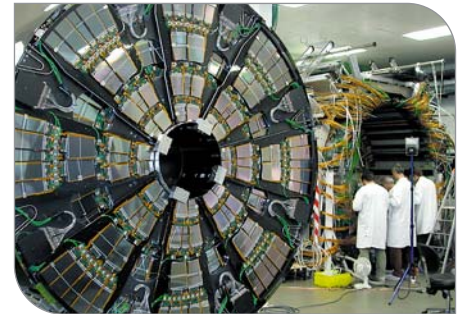
Construction of the CMS silicon strip detector, with KIT providing a major share.
