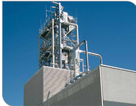
Fast pyrolysis in the bioliq ® plant: Biomass is converted into a liquid intermediate product for transportation.
